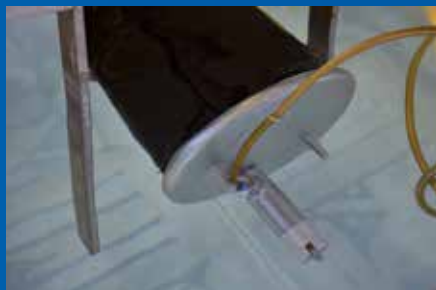
Total leakage monitoring in the water tank under 1.0–1.5 bar air pressure
