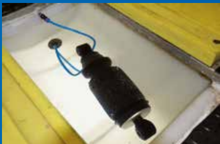
Total leakage monitoring in the water tank under 1.0–1.5 bar air pressure
