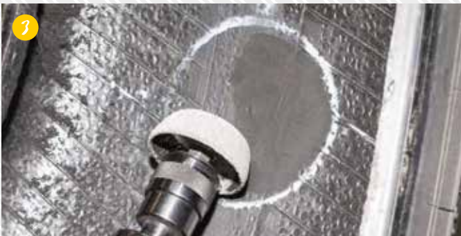
3 Roughen with the rod grinder (order no. 9502 537 401) and vacuum with the compressed air suction gun (order no. 9505 155 090).
