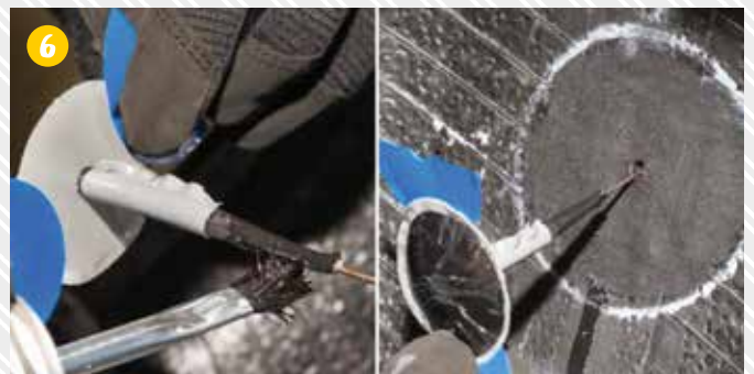
6 Push through the matching repair body.
