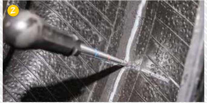
2 Determine the hole size with a pre-cutter (order no. 9503 001 081).
