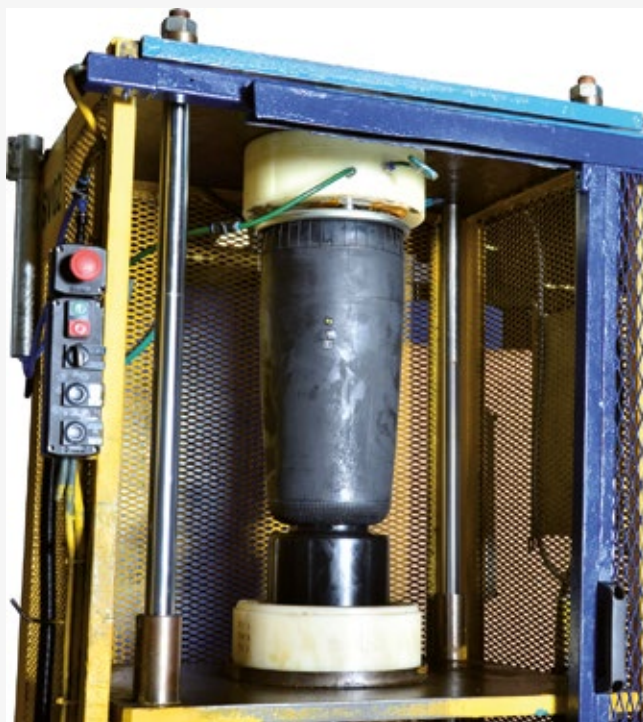
Piston assembly machine - air springs without base plate
