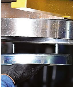
Crimped plate (headplate) is tensioned in the crimping machine (magnetic uptake).
