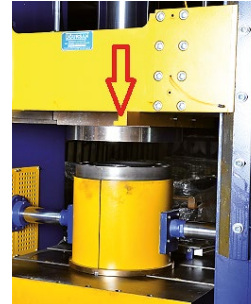
The plate holder moves down and flares the air spring.
