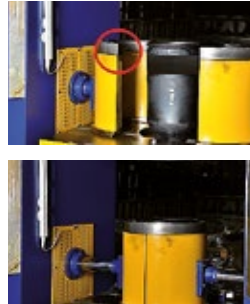
The holding jaws close and the tool prepares the upper cone bead for the process.
