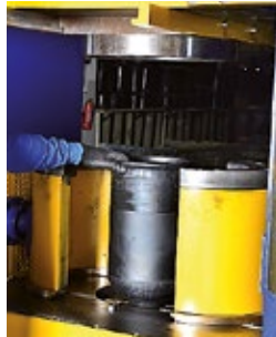
The air spring is put into the press.
