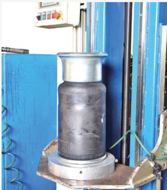
Piston assembly machine - air springs with vulcanised base plate or clamping plate
